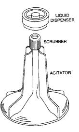
Note: The Liquid Dispenser may be used also for adding liquid detergent with the ULTRA WASH cycle. Dispenser should be cleaned after use of liquid detergent. See p. 8.
