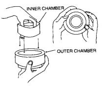
To reassemble, hold both pieces in an upright position. Insert the inner chamber into the outer chamber using ribs to position parts. Rotate until a stop is felt. Push parts together firmly to engage locking tabs.
